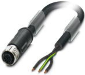
Power cable, 3-position, PVC, black, free cable end, on Socket straight M12, coding: S, cable length: 1 m, for AC current up to 16 A/230 V
