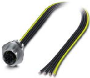
Flush-type connector, Power, 4-position, Socket, M12, S power, Front mounting, M16 x 1.5, Individual wires, cable length: 0.5 m, 1.31 mm 2 , UL/cUL stranded hook-up wire
