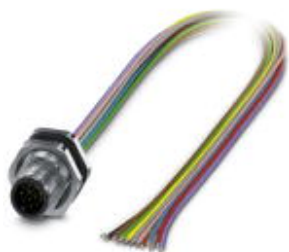
Flush-type connector, Universal, 12-position, Plug, M12, A-coded, Rear mounting, M16 x 1.5, Individual wires, cable length: 0.5 m, 0.14 mm 2 , TPE litz wire
