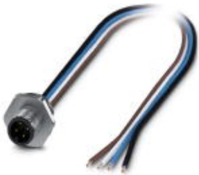
Flush-type connector, Universal, 5-position, Plug, M12, B-coded, Front mounting, M16 x 1.5, Individual wires, cable length: 0.5 m, 0.34 mm 2 , TPE litz wire
