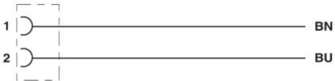
Contact assignment of the DEUTSCH DT06-2S
