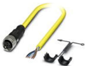
Sensor/actuator cable, 5-position, PVC, yellow, free cable end, on Socket straight M12 SPEEDCON, coding: A, cable length: 2 m
