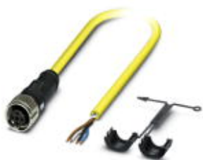
Sensor/actuator cable, 4-position, PVC, yellow, free cable end, on Socket straight M12 SPEEDCON, coding: A, cable length: 2 m
