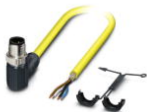
Sensor/actuator cable, 4-position, PVC, yellow, shielded, Plug angled M12 SPEEDCON, coding: A, on free cable end, cable length: 10 m
