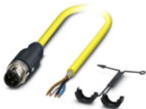
Sensor/actuator cable, 4-position, PVC, yellow, shielded, Plug straight M12 SPEEDCON, coding: A, on free cable end, cable length: 10 m
