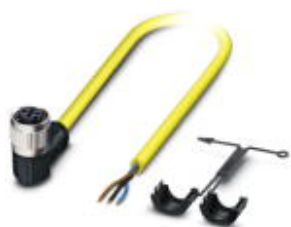
Sensor/actuator cable, 3-position, PVC, yellow, free cable end, on Socket angled M12 SPEEDCON, coding: A, cable length: 10 m
