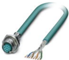
Assembled Ethernet cable, shielded, 4-pair, AWG 26 stranded (7-wire), RAL 5021 (sea blue), M12 flush-type socket, rear/screw mounting with M16 thread to free cable end, line, length 5 m
