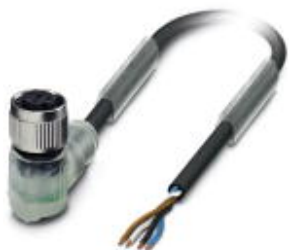
Sensor/actuator cable, 4-position, PUR halogen-free, black-gray RAL 7021, free cable end, on Socket angled M12 SPEEDCON, coding: A, with 3 LEDs, cable length: 1.5 m
