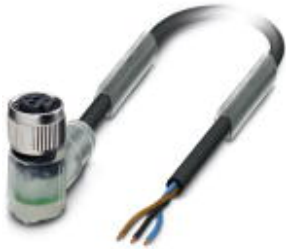
Sensor/actuator cable, 3-position, PUR halogen-free, black-gray RAL 7021, free cable end, on Socket angled M12 SPEEDCON, coding: A, with 2 LEDs, cable length: 1.5 m
