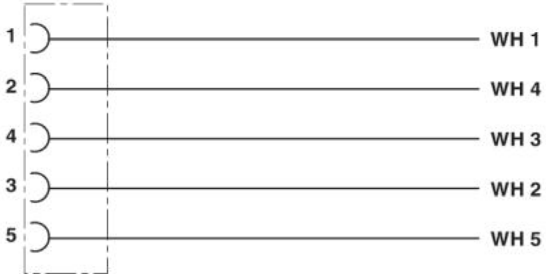
Contact assignment of the M12 socket
