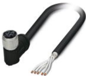
Sensor/actuator cable, 5-position, PE-X halogen-free, black, shielded, free cable end, on Socket angled M12 SPEEDCON, coding: A, cable length: 10 m, For railway applications
