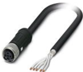
Sensor/actuator cable, 5-position, PE-X halogen-free, black, shielded, free cable end, on Socket straight M12 SPEEDCON, coding: A, cable length: 2 m, For railway applications
