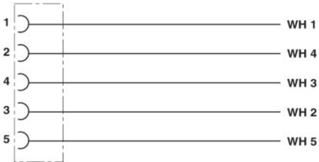
Contact assignment of the M12 socket
