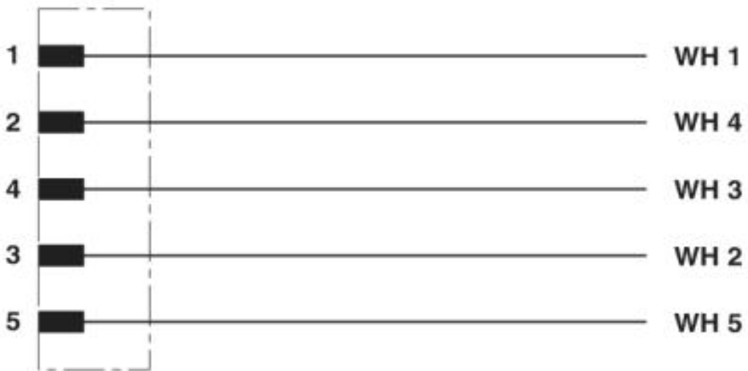
Contact assignment of the M12 plug
