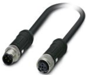
Sensor/actuator cable, 4-position, PE-X halogen-free, black, shielded, Plug straight M12 SPEEDCON, coding: A, on Socket straight M12 SPEEDCON, coding: A, cable length: 5 m, For railway applications
