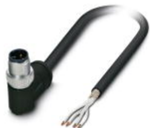
Sensor/actuator cable, 4-position, PE-X halogen-free, black, shielded, Plug angled M12 SPEEDCON, coding: A, on free cable end, cable length: 5 m, For railway applications
