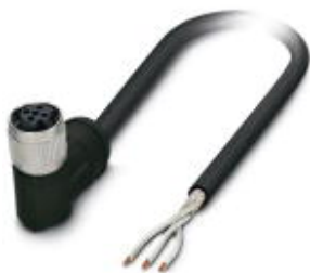
Sensor/actuator cable, 3-position, PE-X halogen-free, black, shielded, free cable end, on Socket angled M12 SPEEDCON, coding: A, cable length: 10 m, For railway applications
