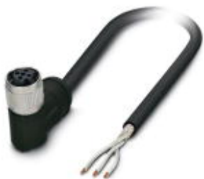
Sensor/actuator cable, 3-position, PE-X halogen-free, black, shielded, free cable end, on Socket angled M12 SPEEDCON, coding: A, cable length: 2 m, For railway applications
