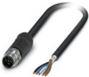
Sensor/actuator cable, 5-position, PE-X/PE-X halogen-free, black-gray RAL 7021, shielded, Plug straight M12, coding: A, on free cable end, cable length: 2 m, for outdoor applications, with high-grade steel knurl
