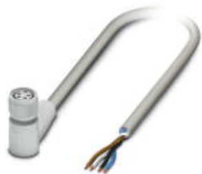
Sensor/actuator cable, 4-position, PP-EPDM halogen-free, gray RAL 7035, free cable end, on Socket angled M8, with 2 LEDs, cable length: 5 m, Hygienic design, with plastic knurl
