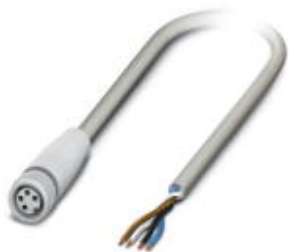
Sensor/actuator cable, 4-position, PP-EPDM halogen-free, gray RAL 7035, free cable end, on Socket straight M8, cable length: 3 m, Hygienic design, with plastic knurl
