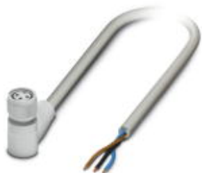
Sensor/actuator cable, 3-position, PP-EPDM halogen-free, gray RAL 7035, free cable end, on Socket angled M8, with 2 LEDs, cable length: 10 m, Hygienic design, with plastic knurl
