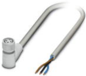
Sensor/actuator cable, 3-position, PP-EPDM halogen-free, gray RAL 7035, free cable end, on Socket angled M8, with 2 LEDs, cable length: 5 m, Hygienic design, with plastic knurl
