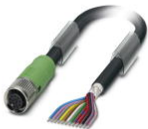
Sensor/actuator cable, 12-position, PUR/PVC, black RAL 9005, shielded, free cable end, on Socket straight M12 SPEEDCON, coding: A, cable length: 20 m
