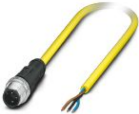
Sensor/actuator cable, 3-position, PVC, yellow, Plug straight M12 SPEEDCON, coding: A, on free cable end, cable length: 10 m
