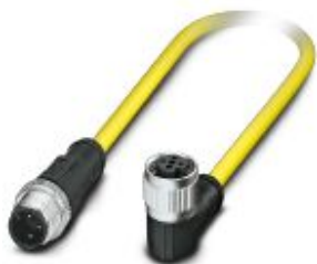
Sensor/actuator cable, 3-position, PVC, yellow, Plug straight M12 SPEEDCON, coding: A, on Socket angled M12 SPEEDCON, coding: A, cable length: 0.5 m
