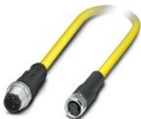
Sensor/actuator cable, 3-position, PVC, yellow, Plug straight M12, coding: A, on Socket straight M8, cable length: 0.5 m
