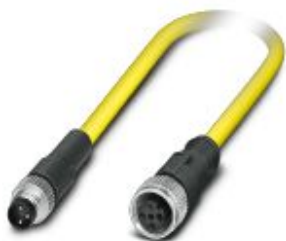
Sensor/actuator cable, 3-position, PVC, yellow, Plug straight M8, on Socket straight M12, coding: A, cable length: 1.5 m
