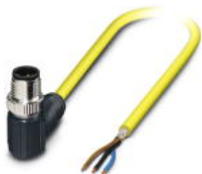
Sensor/actuator cable, 3-position, PVC, yellow, shielded, Plug angled M12 SPEEDCON, coding: A, on free cable end, cable length: 10 m
