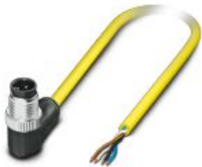
Sensor/actuator cable, 4-position, PVC, yellow, Plug angled M12 SPEEDCON, coding: A, on free cable end, cable length: 2 m
