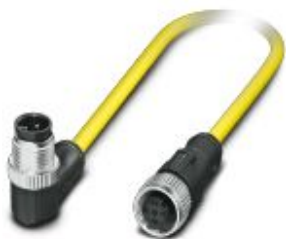
Sensor/actuator cable, 4-position, PVC, yellow, Plug angled M12 SPEEDCON, coding: A, on Socket straight M12 SPEEDCON, coding: A, cable length: 0.5 m
