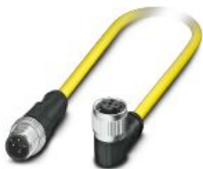
Sensor/actuator cable, 4-position, PVC, yellow, Plug straight M12 SPEEDCON, coding: A, on Socket angled M12 SPEEDCON, coding: A, cable length: 0.5 m
