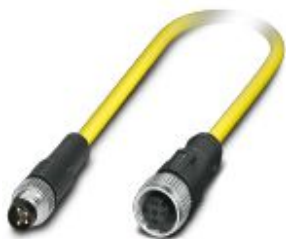
Sensor/actuator cable, 4-position, PVC, yellow, Plug straight M8, on Socket straight M12 SPEEDCON, coding: A, cable length: 1.5 m
