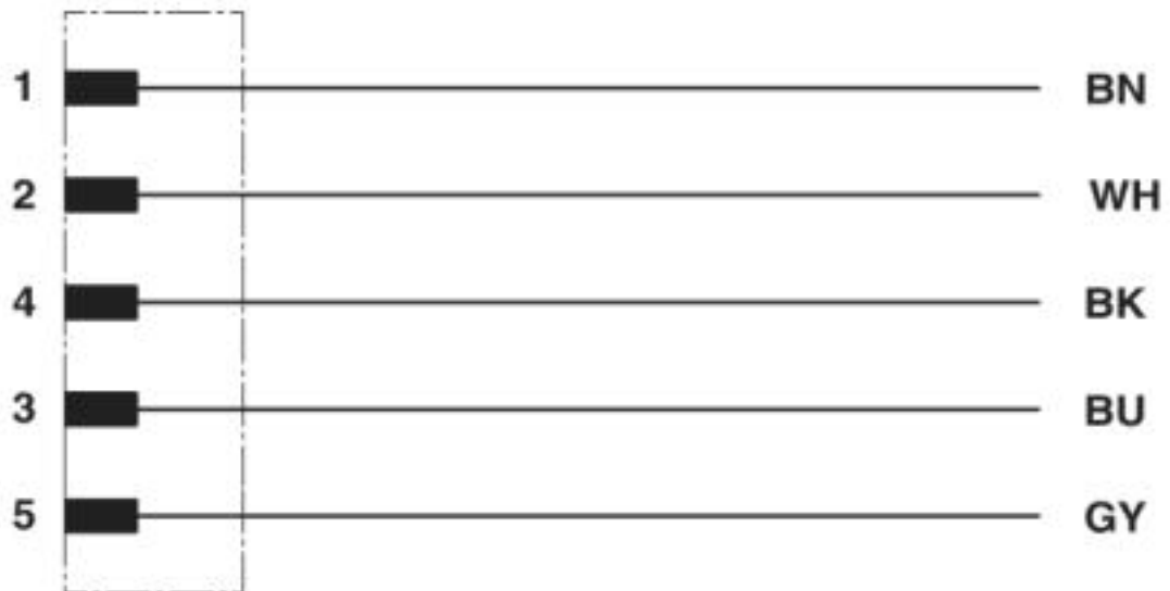
Contact assignment of the M12 plug
