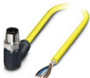
Sensor/actuator cable, 5-position, PVC, yellow, shielded, Plug angled M12 SPEEDCON, coding: A, on free cable end, cable length: 5 m
