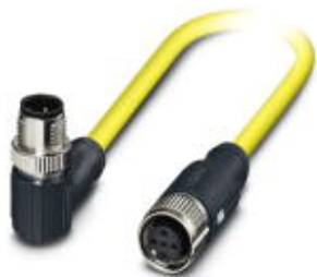
Sensor/actuator cable, 5-position, PVC, yellow, shielded, Plug angled M12 SPEEDCON, coding: A, on Socket straight M12 SPEEDCON, coding: A, cable length: 0.5 m
