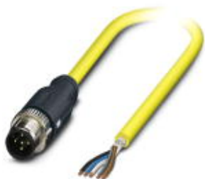
Sensor/actuator cable, 5-position, PVC, yellow, shielded, Plug straight M12 SPEEDCON, coding: A, on free cable end, cable length: 2 m
