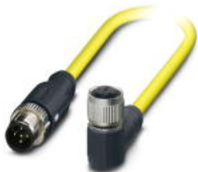
Sensor/actuator cable, 5-position, PVC, yellow, shielded, Plug straight M12 SPEEDCON, coding: A, on Socket angled M12 SPEEDCON, coding: A, cable length: 0.5 m
