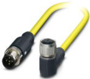
Sensor/actuator cable, 5-position, PVC, yellow, shielded, Plug straight M12 SPEEDCON, coding: A, on Socket angled M12 SPEEDCON, coding: A, cable length: 1.5 m
