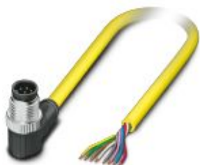
Sensor/actuator cable, 8-position, PVC, yellow, Plug angled M12 SPEEDCON, coding: A, on free cable end, cable length: 2 m
