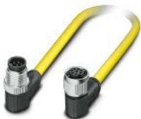
Sensor/actuator cable, 8-position, PVC, yellow, Plug angled M12 SPEEDCON, coding: A, on Socket angled M12 SPEEDCON, coding: A, cable length: 0.5 m
