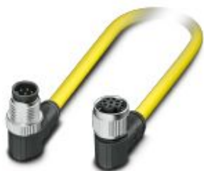
Sensor/actuator cable, 8-position, PVC, yellow, Plug angled M12 SPEEDCON, coding: A, on Socket angled M12 SPEEDCON, coding: A, cable length: 1.5 m
