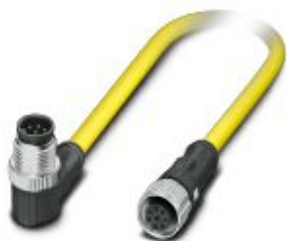
Sensor/actuator cable, 8-position, PVC, yellow, Plug angled M12 SPEEDCON, coding: A, on Socket straight M12 SPEEDCON, coding: A, cable length: 0.5 m
