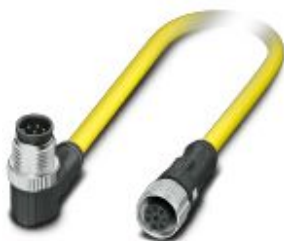
Sensor/actuator cable, 8-position, PVC, yellow, Plug angled M12 SPEEDCON, coding: A, on Socket straight M12 SPEEDCON, coding: A, cable length: 1.5 m
