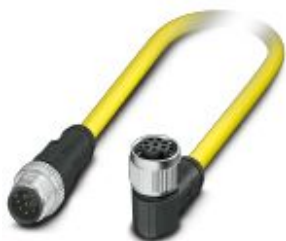
Sensor/actuator cable, 8-position, PVC, yellow, Plug straight M12 SPEEDCON, coding: A, on Socket angled M12 SPEEDCON, coding: A, cable length: 1.5 m
