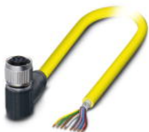
Sensor/actuator cable, 8-position, PVC, yellow, shielded, free cable end, on Socket angled M12 SPEEDCON, coding: A, cable length: 2 m
