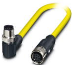
Sensor/actuator cable, 8-position, PVC, yellow, shielded, Plug angled M12 SPEEDCON, coding: A, on Socket straight M12 SPEEDCON, coding: A, cable length: 1.5 m
