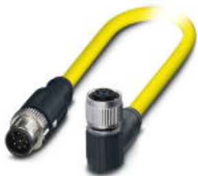
Sensor/actuator cable, 8-position, PVC, yellow, shielded, Plug straight M12 SPEEDCON, coding: A, on Socket angled M12 SPEEDCON, coding: A, cable length: 0.5 m
